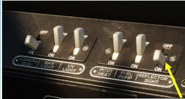
1 Reflector Gunsight Power Switch • DOWN: ON • UP: OFF
