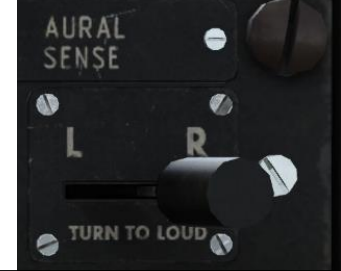
Loop Antenna at 040 Switch RIGHT No Sound Audible No need to turn antenna RIGHT
