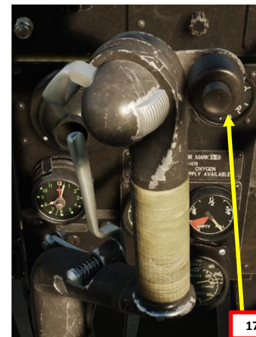
Bomb Release & Gun Camera (Guncam) Button • RSHIFT+SPACE The function of the button depends of the position of the Bombs or Camera Changeover Switch
