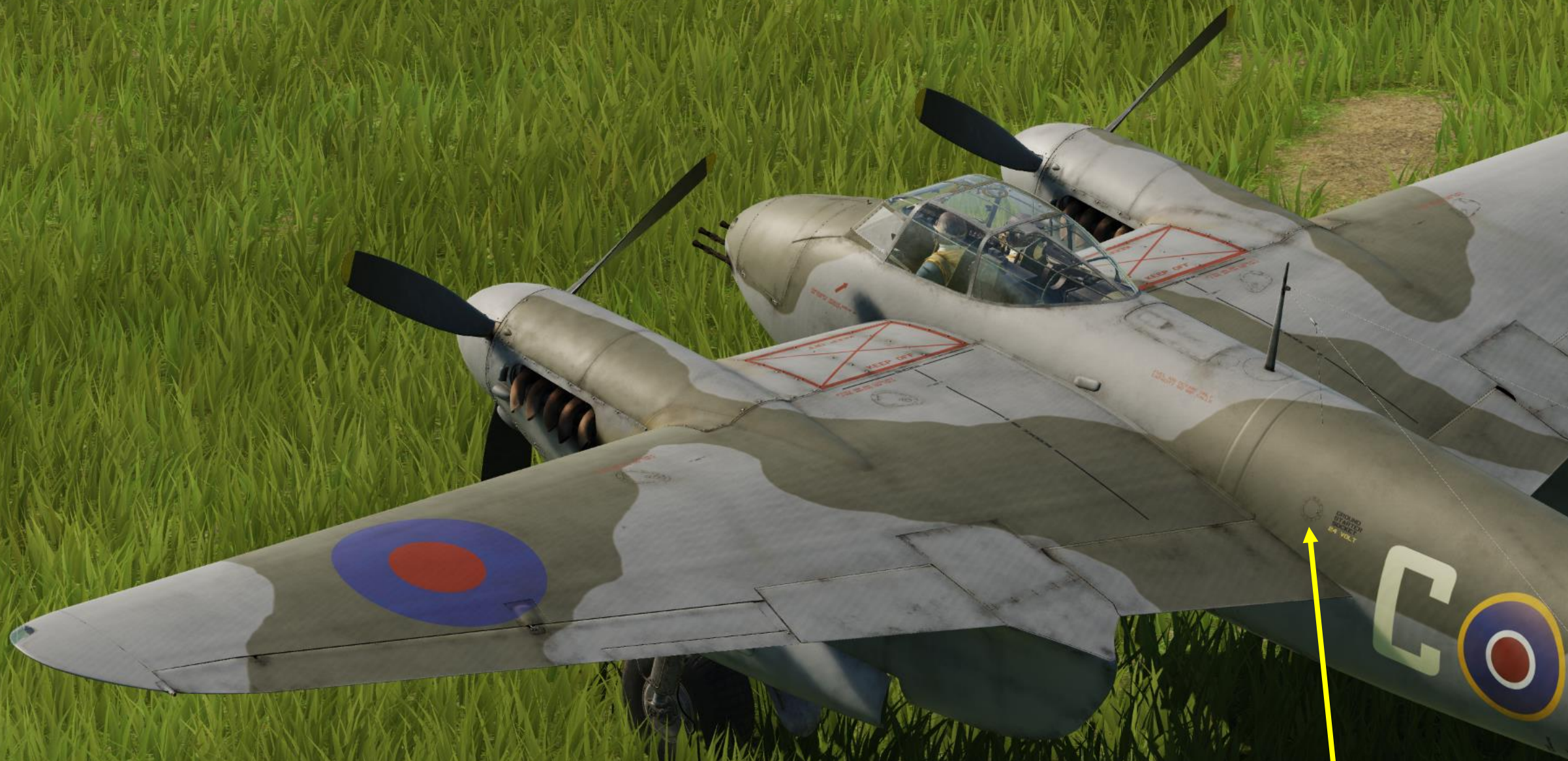
Ground Power Socket (24 Volts)
